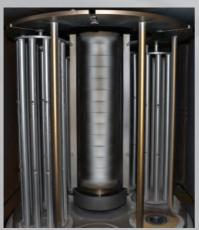
Segmented TiB<sub>2</sub>-cathode for SCIL<sup>®</sup>-Technology
