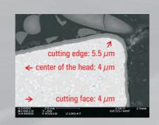
Thickness measured by Calotest at center of the head Cutting face
