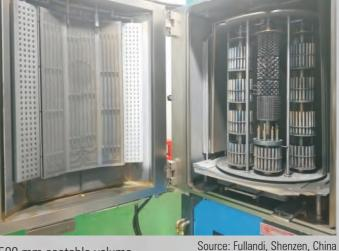
Machines with 2 sputtering cathodes, DC and HIPIMS modes ø550x500 mm coatable volume. Many moving parts in the machinery and automotive industries do not need extra hard coatings. The most important requirements are:
