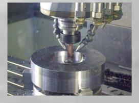
Carbide End Mills Ø10mm, z=4, steel 34CrNiMo6 (30 HRC), Coolant: MQL; Minimum lubrication - Tested tools: 2x4 Source: Carmex, Maalot, IL
