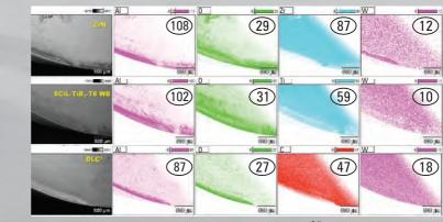
**X** EDX- detection frequency of the respective element: DLC<sup>3®</sup> deposited by  $\pi$ 211 SEM and EDX after 283 m tool life Material: 3.4365 AlZnMgCu1,5 - Tool: Torus end mill Ø12mm – r=2.5mm – z=2 vc=377 m/min – ae=5mm – ap=6mm – fz=0.2 mm/rev
