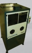
CB411 and CB1011 For *π*<sup>411</sup>, *π*<sup>1511</sup>, and *PL*<sup>1011</sup> Safe cooling of the tools immediately after coating.
