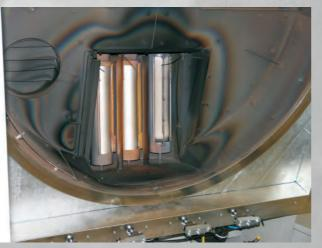
Three rotating cathodes for flexible deposition
