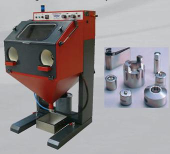
The PolishPeen 770 equipment is a vacuum blasting cabin with an injector in the blasting pistol. A special media is used as polishing powder.
