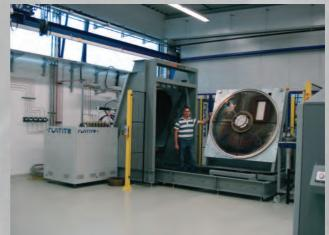
Saw band coils up to 1.4 m diameter can be coated. The back side of the saw band is deposited with a help of a planar target.
