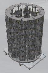
10 axis carousel for hobs and gearboxes D=143 mm
