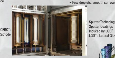
Sputter-Technology: SCIL<sup>®</sup> : • **Sputter Coatings** Induced by LGD<sup>®</sup> LGD<sup>®</sup>: Lateral Glow Discharge
