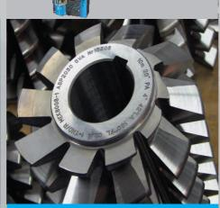
Coating for hobbing in the eco machines  $\pi^{\text{Gall}}$  eco cathodes: CrTi-LARC - Al-LARC - Cr-LARC Stoichiometry: CrN - AlCrN-G - AlCrTiN-NL • for hobs with big diameters
