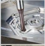
183 🛛 VBave 📃 VBmax 180 160 140 120 102 97 100 86 72 80 67 60 60 44 40 20 0 TiXCo<sup>3®</sup> nACRo<sup>3®</sup> AITiN (market) AlTiN + AlCrN (market) Torus end mill in cold-working steel X210Cr12 (1.2080) - 61.5 HRCØ 8 mm - z=4 - ap=0.1mm - ae=3mm vc=100m
