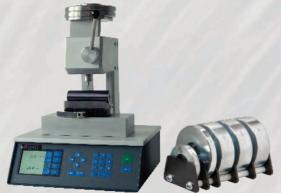
Scratch tester with constant loads for testing in production (go or not go) Source: BAQ, Braunschweig, Germany
