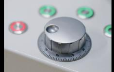
A thumbwheel positioned to the right of the operator activates the digitized axes, such as the table, the spindle and the expansion system, for easy adjustments.
