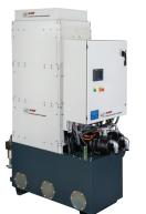
The Chipblaster V2-80 can operate as two completely independent 40 liter (10 gpm) modules or combine to provide high pressure and very high volumes 80 liters at any time during the same program.
