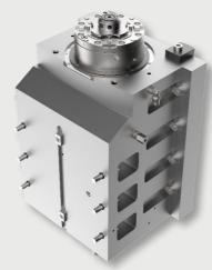
The 3-axis **E-80-CNC** unit meets the most common needs: drilling, milling, reaming and tapping. It can be equipped with two spindles and installed horizontally or vertically. This unit can also be used on the *imo-compact* and the *imo-space*.
