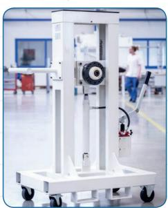
The grinding wheel trolley is used to pick-up and transport the flange-mounted wheels from the set-up station to the grinding machine. It has two fixed and two steerable castors for flexible movement, and is manually operated.
