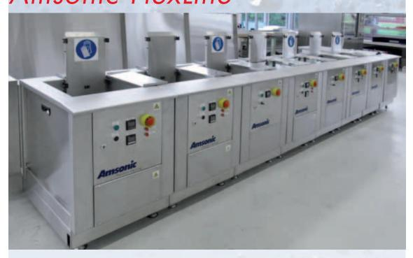
FlexLine is a water-based, modular ultrasonic batch cleaning system. Units can be added to or removed from the system flexibly to meet your precise cleaning requirements. Designed to be easily assembled, FlexLine allows versatility in process customisation for all your needs. It also offers exceptional value for money while remaining a customized solution. The user can retrofit additional modules to keep up with the various cleaning demands, thus creating the complete batch cleaning system.
